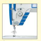
按鍵倒縫,補針,LED燈,三合一,使用輕鬆。 With back-tacking, second stitch and LED light three-in-one function for easy operation
